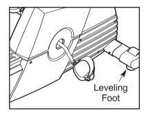
slightly during use, turn one or both of the leveling feet under the front stabilizer until the rocking motion is eliminated.
